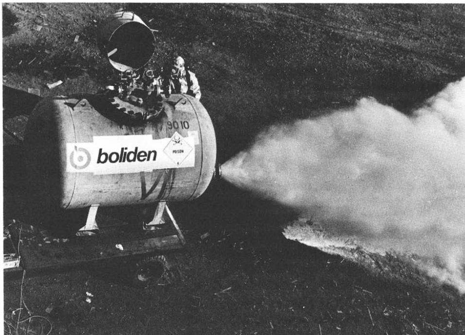
Fig. 1. The test tank in operation. The valve is operated manually to achieve short opening and closing times.
